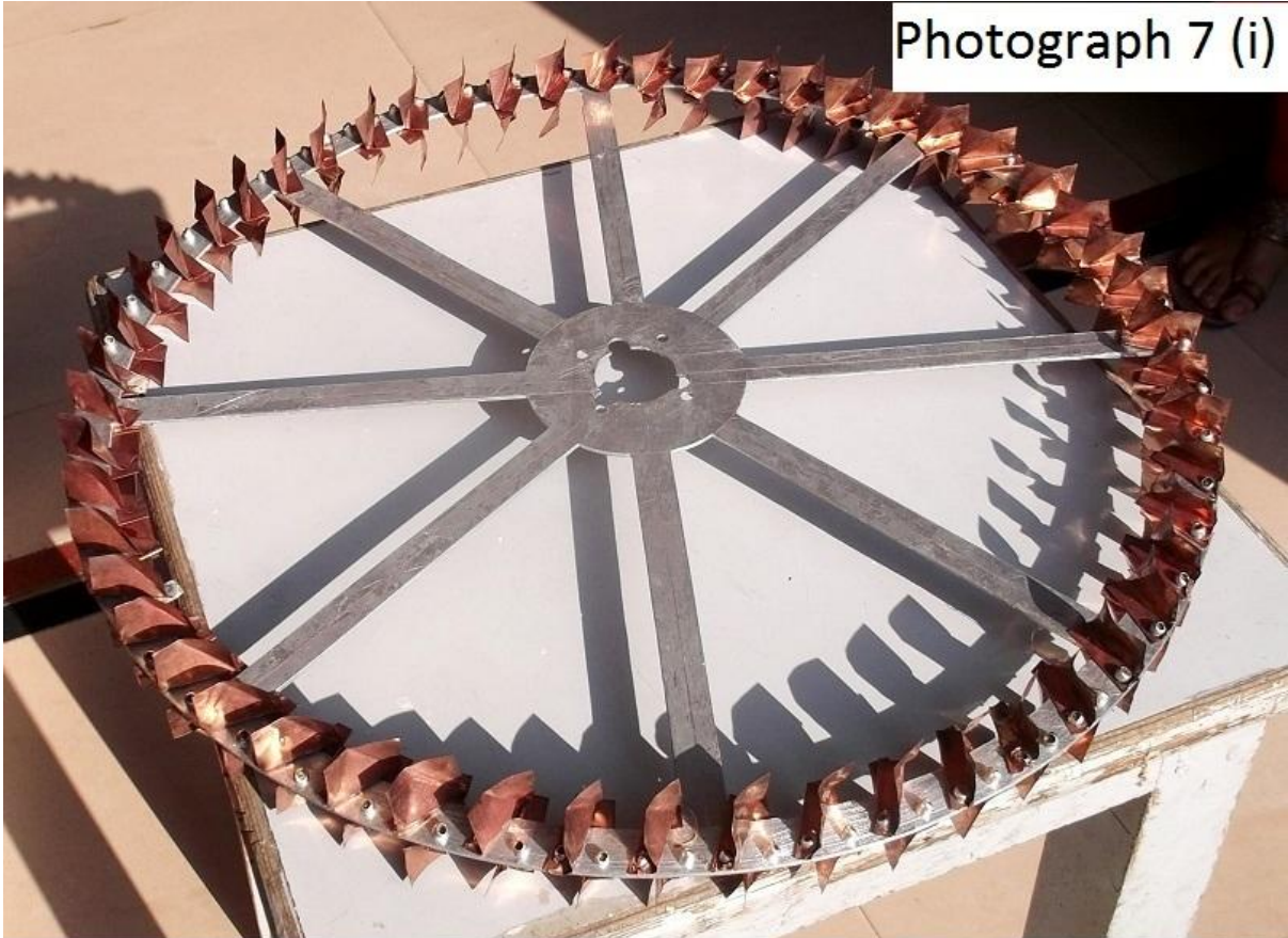
Aluminium Wheel/Impeller - cut to design, Copper sheet fins attached onto the Aluminium Wheel/Impeller rim, both at the top and at the bottom.
