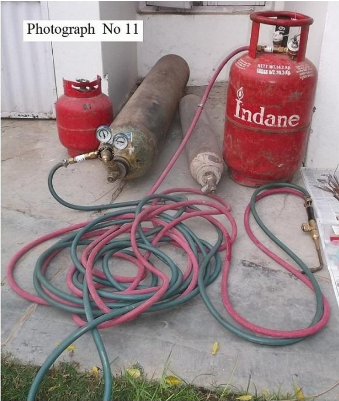
Standard Gas brazing equipment used with gases Oxygen and LPG . Standard LPG Welding Torch and Brazing Gun , as used .
