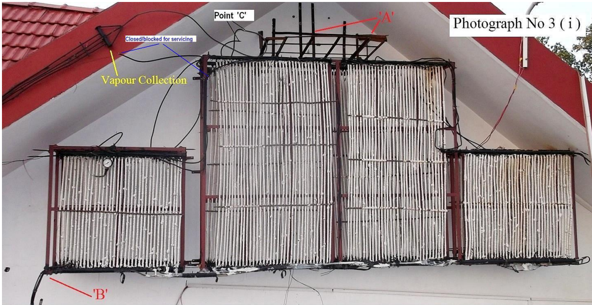
A view of the Cooling Assembly , the base of which is at a height of 18 Feet , above the base of the Heating Assembly . The Copper Tubing is covered with water absorbent cloth. Holder of the Vapour/Gas Turbine is seen at the Top of the Assembly at point 'A' . The entire Cooling Assembly is tilted towards the left at Point 'B' , for the Diethyl ether , in liquid form , to flow back to the base of the Heating Assembly
