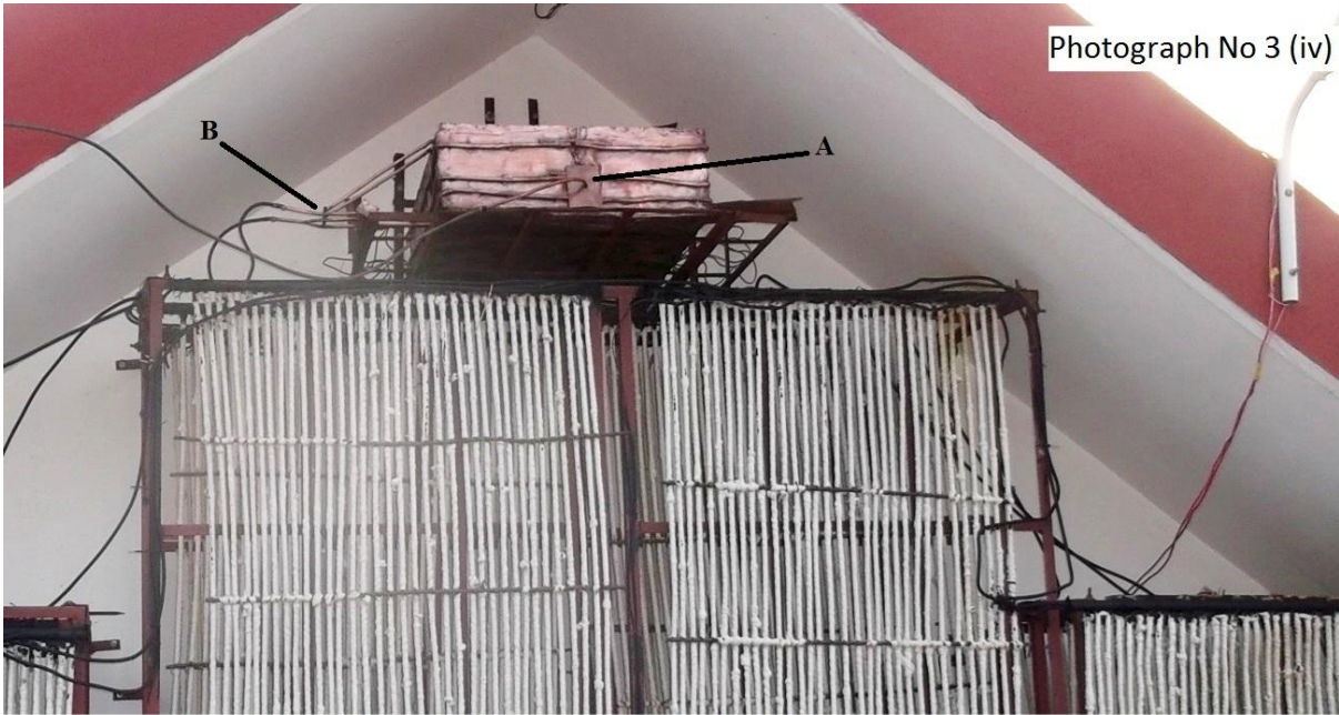
View of Vapour/Gas Turbine showing the Vapour Inlet at Point 'A' and Working Fluid outlet at Point 'B' .
