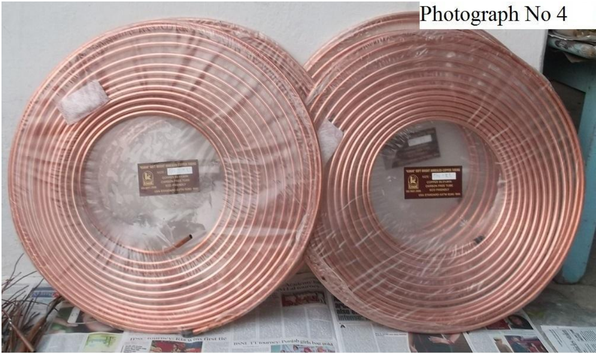
Copper pipes / rolls – Copper Tubing , pure Copper 99.9 % , I.D. 6.6 mm O.D 7.8 mm . Standard tubing used in fabricating the Heating Assembly and Cooling Assembly .
