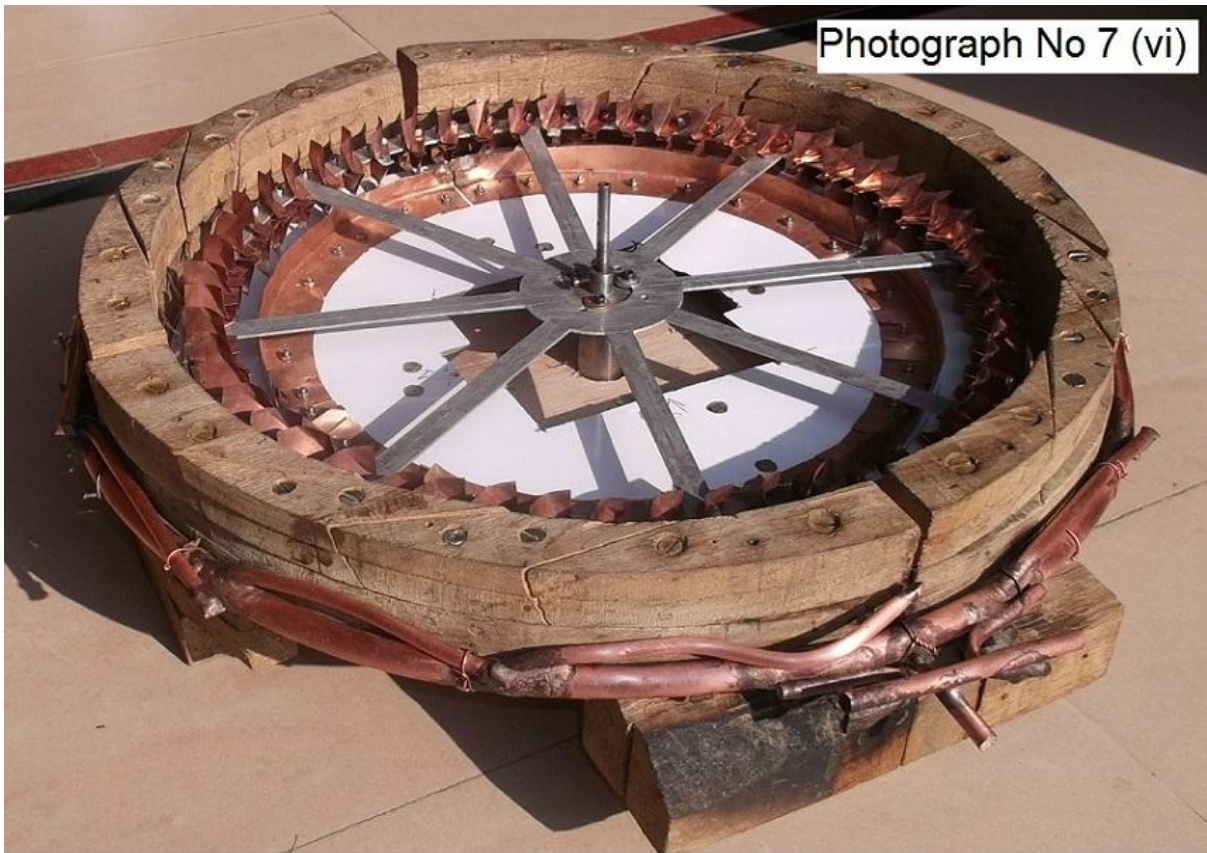
Vapour/Gas Turbine with Aluminium Wheel/Impeller and Generator/Dynamo affixed in place.
