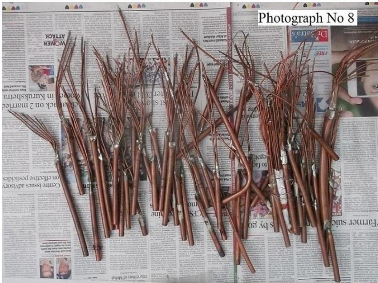
Combinations of jets/nozzles for the working of the Vapour/Gas Turbine. The copper capillary tubes are tipped with cut pieces from Hypodermic needles .
